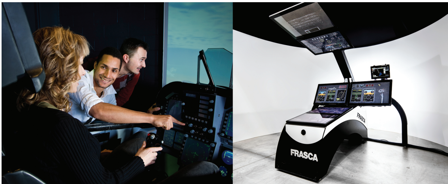
Figure 9-4. A level 4 FTD used for procedure training.
